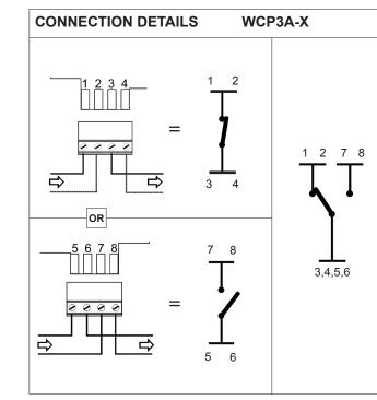
X in the WCP code (above) represents the final digits of the part number, which indicate MCP colour, component values, mounting options and element type. eg WCP1A -R470SF = (WCP1A, Red, 470R, Surface, Flexible Element).
