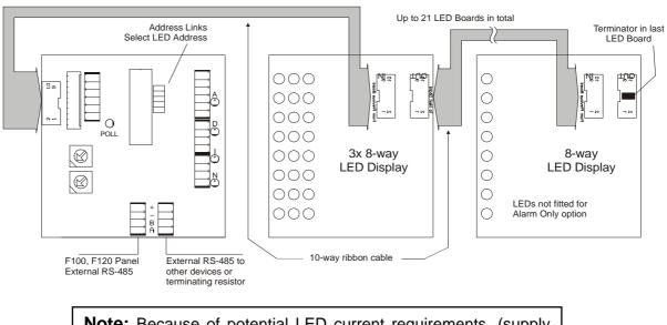
**Note:** Because of potential LED current requirements, (supply current is 500mA), it is recommended that a maximum of 12 AFI boards be connected to one AFI Controller.
