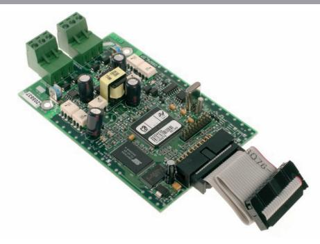
The VESDAnet™ Interface Card (VN Card) is a simple interface card for the range of VESDA VLF smoke detectors. The VN Card provides seamless VESDAnet communication from the detector to other VESDAnet devices, including configuration and monitoring tools.
