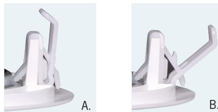
The "Rat-Trap" utilises a spring latching system. Each latch is set like a rat trap before installation into the speaker hole (picture A). When the speaker is pushed into the ceiling, the latches spring open, securing the speaker in place (picture B).
