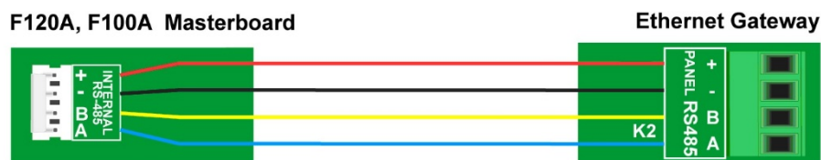
Typical RS485 Wiring Connection to Pertronic AA Control Panel
