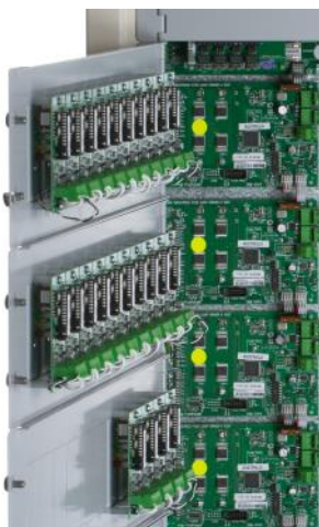
Inside an F220 showing fan controls (left) and loop driver boards.
