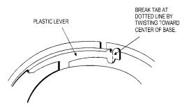
ant tab before installing the detector (see Figure 3A). The tamper-resistant tab is on the detector mounting base. To remove a tamper-resistant detector from the base, use a pocket screwdriver, or similar tool, to depress the tamper-resistant tab and turn the detector counterclockwise. The tab is accessible through the slot on the mounting base (see Figure 3B).
