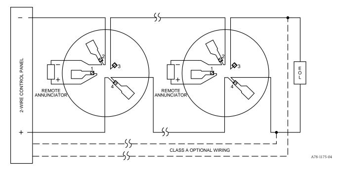
erly wired and mounted to an electrical box, make sure that the shorting spring is in contact with terminal 3. This temporary connection permits the wiring of the loop to be checked for continuity before installation of the detector heads. The shorting spring in the base automatically disengages when the detector head is removed from the base. DO NOT remove the shorting spring since it reengages as the detector head is turned in the base, completing the circuit.
