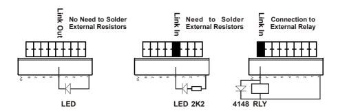
Note: Each 10-way IDC connector may be connected to a mix of Relays and LEDs as required for the application
