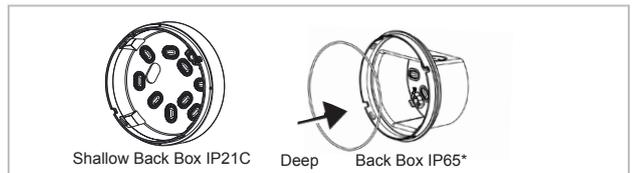
**(ENG)** If the Deep IP65 option is used, the O-ring seal must be fitted as shown. If required, the deep back box gasket accessory can be installed between the back box and the mounting surface. \*IP33C is certified by LPCB to EN54-3 and EN54-23. IP65 is certified by UKAS Accredited test facility.
