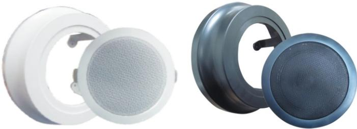
Full-range 4" ceiling loudspeaker, which features five power taps at 100V line for 6W, 3W, 1.5W, 0.75W and 0.375W outputs. An optional surface mount box is available for solid ceiling or wall installation.
