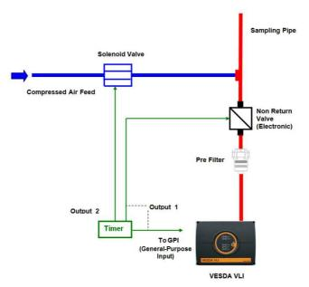
Figure 7 – Automatic back flushing system
