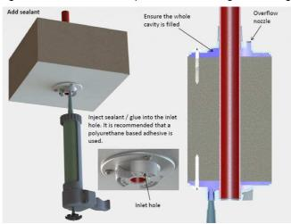
Figure 4 – Applying sealant
