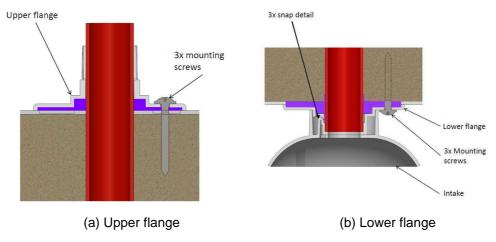
Figure 2 – Components of the sampling kit
